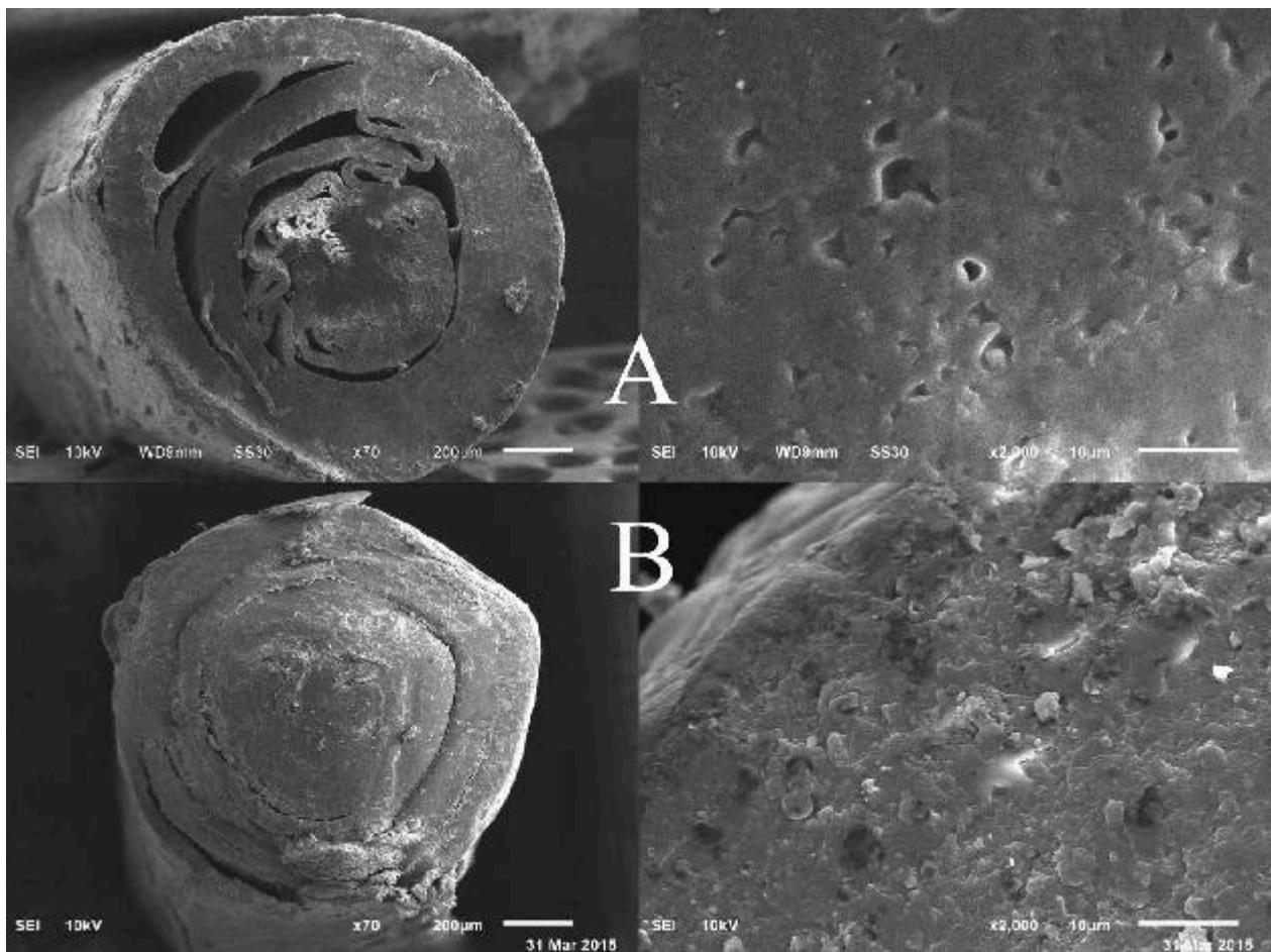
**Figure 3(a).** The Zr-Al-Si post without calcination using 1% chitosan and 8% PMMA matrix.
