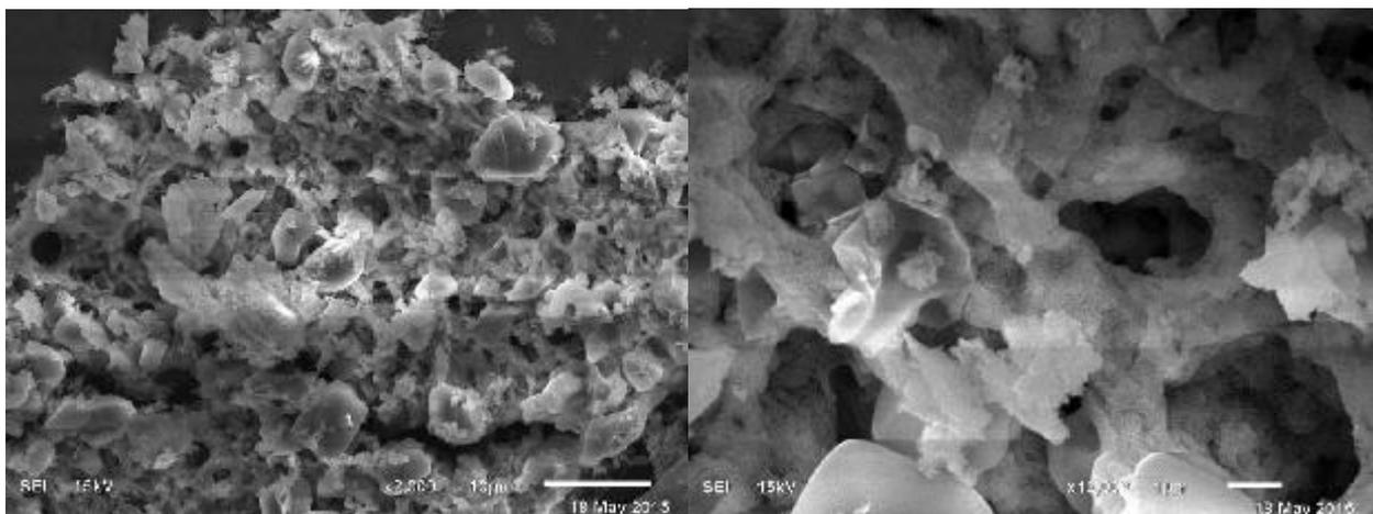
**Figure 1.** The Zr-Al-Si nanoparticle products through calcination templated by ESM.
